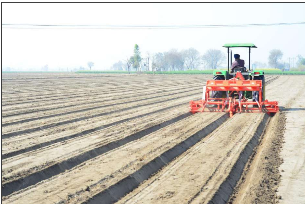
Fig:-6. Multi crop bed planter perform both bed preparation and bed planting
