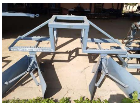
(b) Double row trenchers
