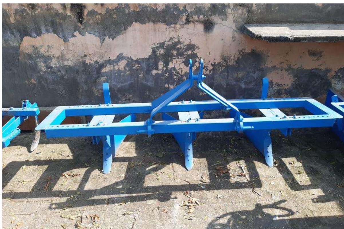
Fig:- 2. Lazer mainly used sugarcane/potato and maize sowing to prepare ridge and furrow
