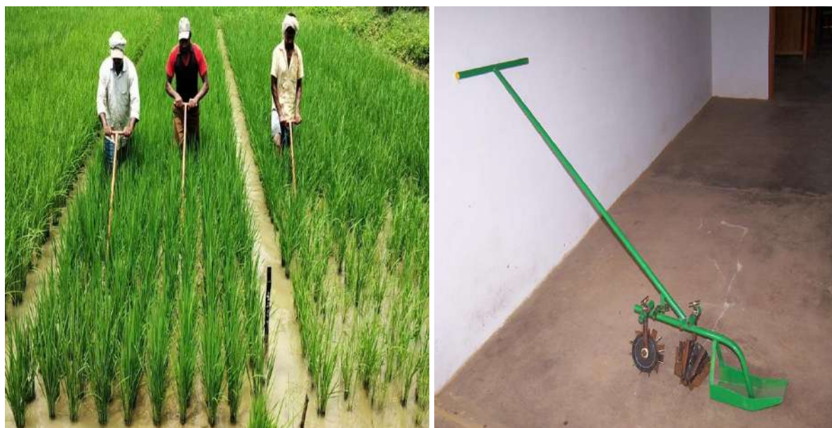
Fig 8. Rotatory conoweeder in rice field
